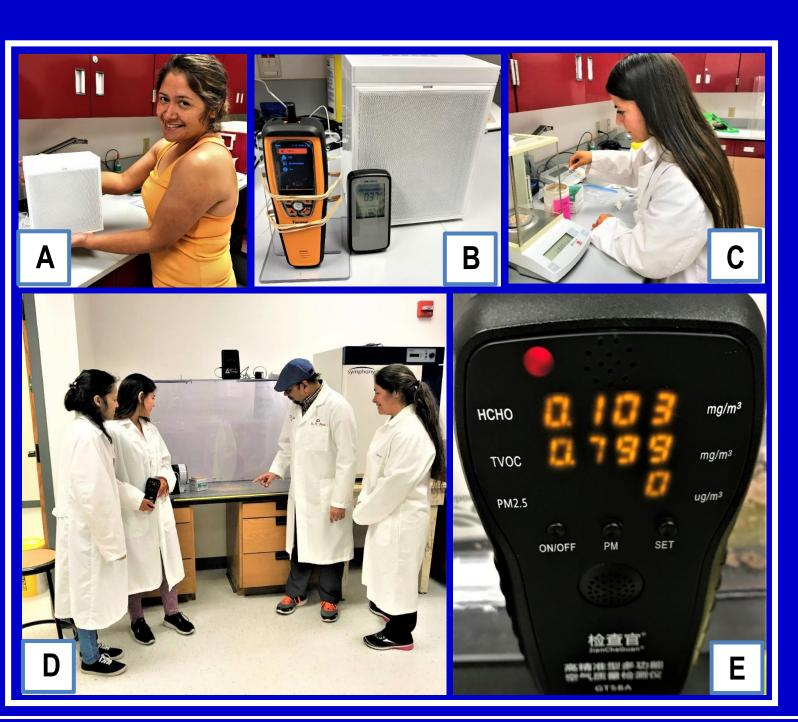
Fig.5. Steps of testing the *i-Adapt* unit: A. *i-Adapt* unit. B & E. Meters for reading HCHO, Total VOC and PM 2.5. C. Weighing the Particulate Matter. B. PM 2.5 testing dust. D. Uniform spreading of the Particulate Matter in the AO Fiberglass chamber by using 4 fans on each 4 corners of the AO chamber. E. Meter readings.
