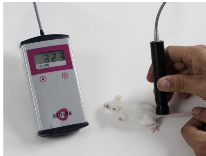
Thermometer with rectal probe to measure body temperature
