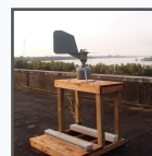
Parapet around roof requires platform to elevate the orifice above the wall
